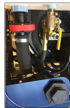
Ports for easy connection to a larger water-tank
